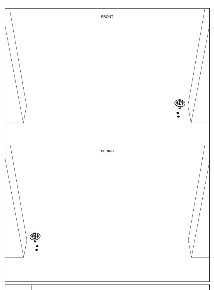
ZENITH SC2 - PERFORATE AND ANCHOR THE BOTTOM ACCESSORY INTO THE FLOOR
