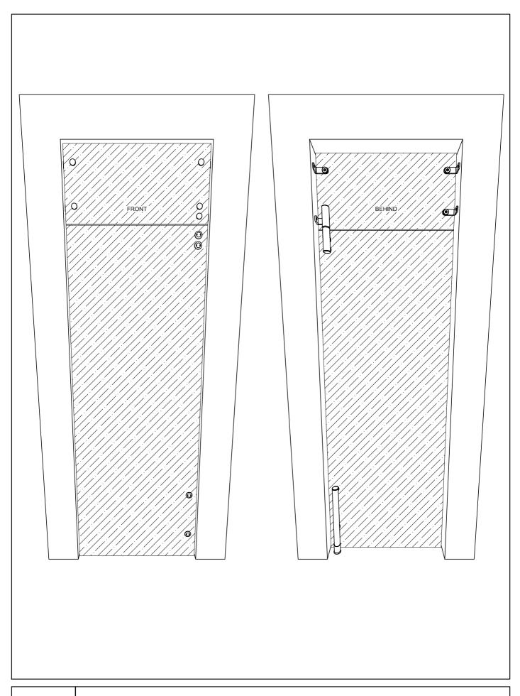
ZENITH SC2 - INSTALL THE REMAINING ACCESSORIES OF THE DOOR CLOSER AND THE WALL BRACKETS
